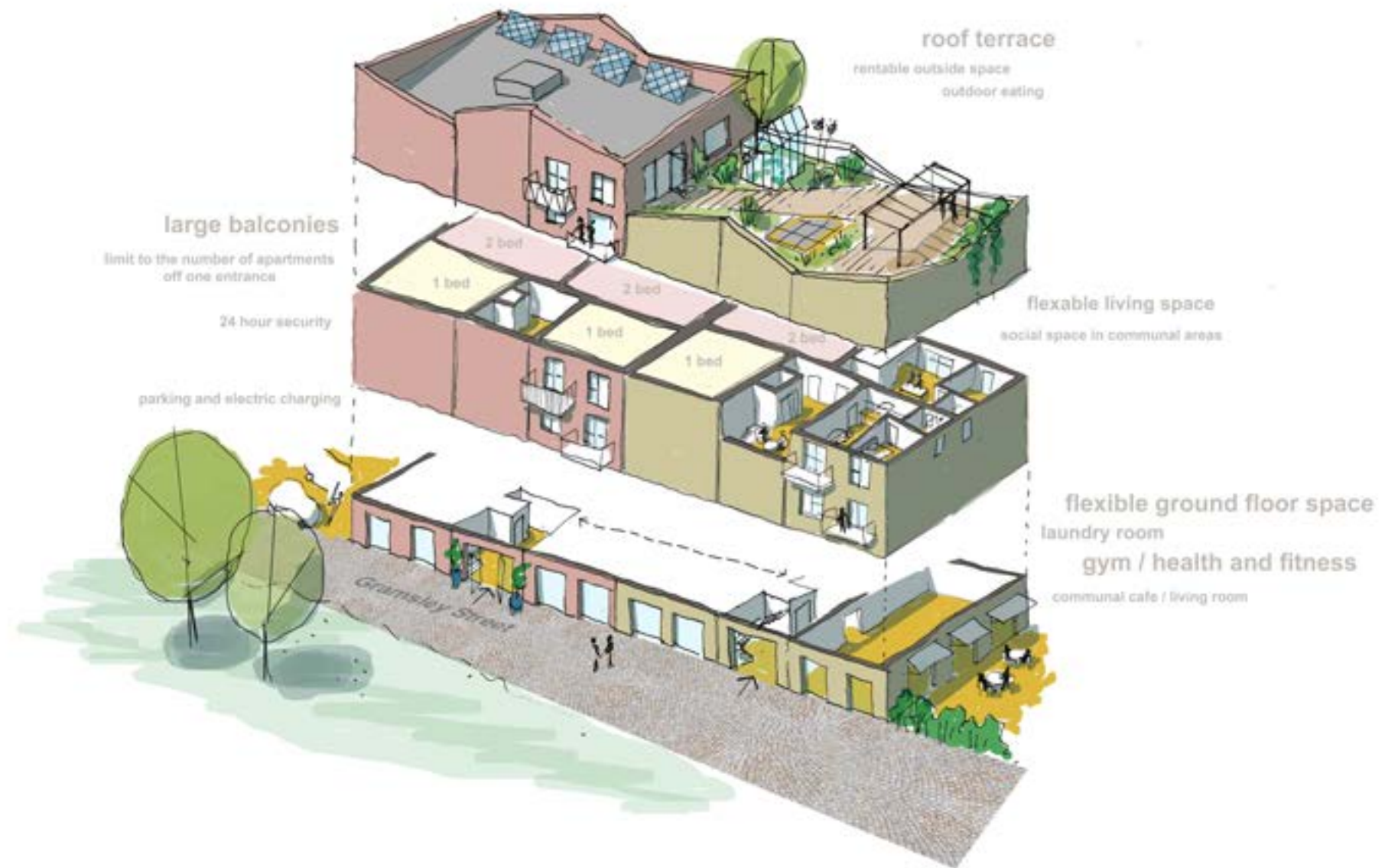
An Intergenerational apartment block which provides one and two bed apartments with shared communal facilities at ground floor with gym, cafe and communal roof garden where over 55's and younger people can live in the same building and share spaces and facilities provided.
